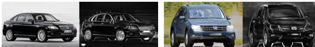
Figure 6.9: Standard deviation of 100 images with the same seed, showing that the random noise mostly affect the edges, the number plates, the wheels and the car logos.
