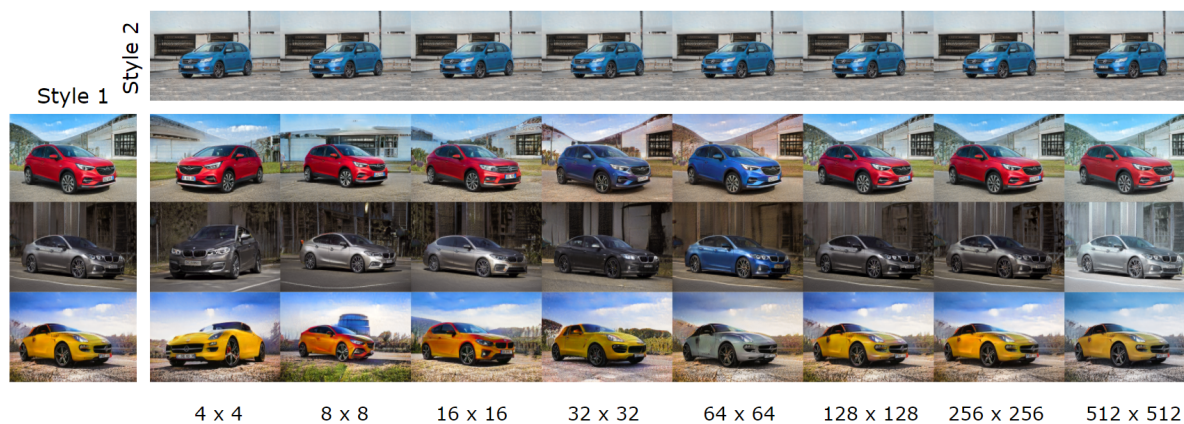
Figure 6.10: Generator output when exchanging the latent vector of style 1 with the latent vector of style 2 for one resolution block. Earlier layers of the generator ( 4 \times 4 - 16 \times 16 ) affect the coarse attributes such as car orientation or shape, while later layers ( 32 \times 32 - 512 \times 512 ) affect small details and colors.
