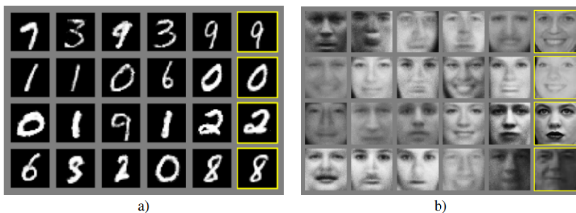
Figure 2.2: Example results of GANs by Ian J. Goodfellow. (a) is trained on the MNIST dataset and (b) is trained on the TFD dataset [Goo+14]. The yellow boxed images display the most similar image from the training dataset to the previous column, to demonstrate that the generator does not simply memorize the training data.
