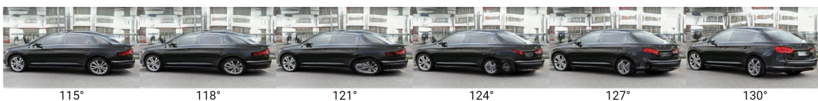
Figure 7.14: An example rotation sequence, where the car tire collapses at 121° similar to previous experiments.
