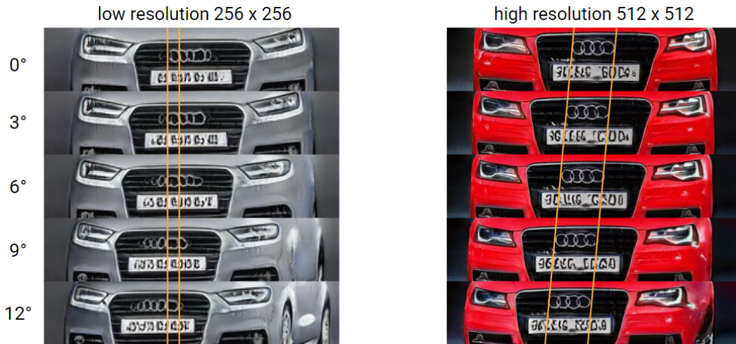
Figure 8.4: A demonstration of the texture sticking effect. It shows that the Audi rings are stuck in place when using the lower resolution, while they move with the car when using the higher resolution.
